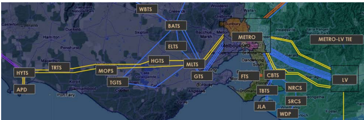
Figure 2 - 500 kV Transmission network backbone
