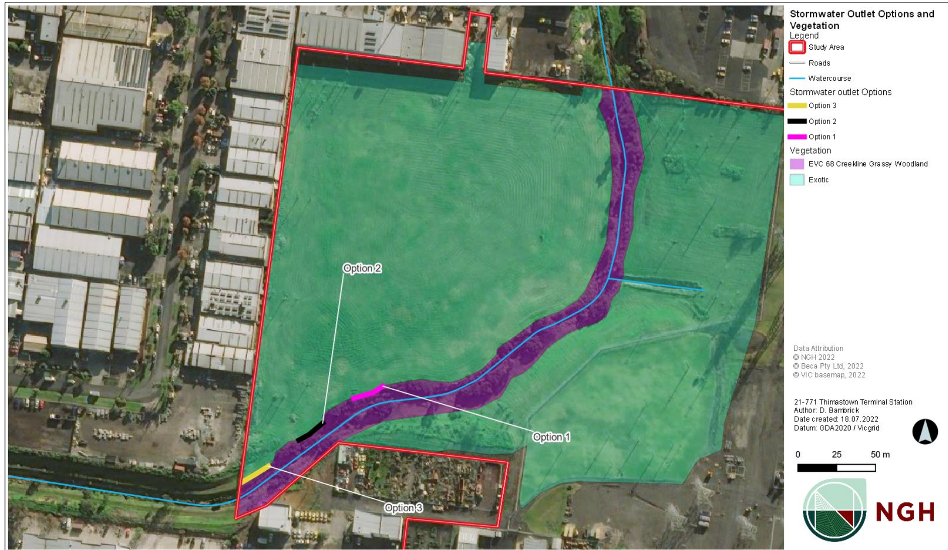
Figure 4-11. Stormwater outlet options
